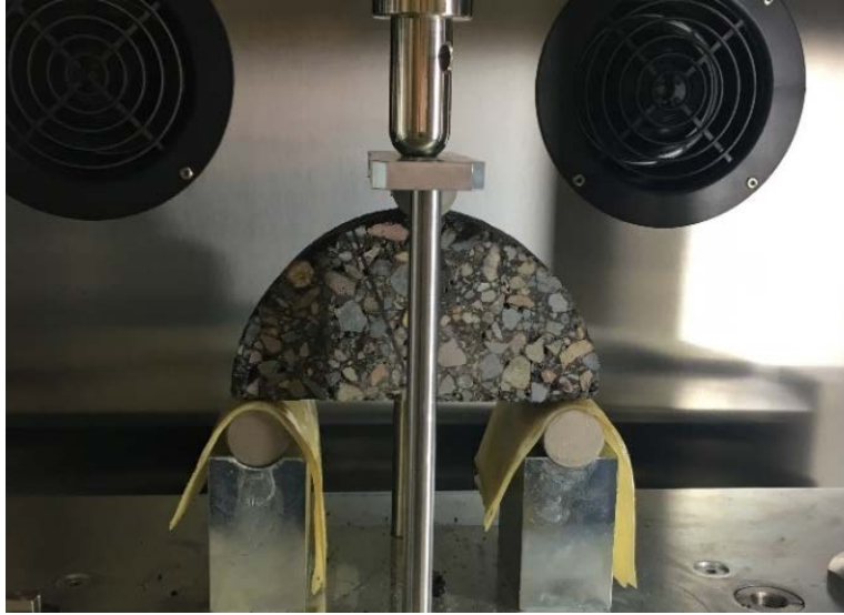
Figure 3.6. SCB loading set up and test
